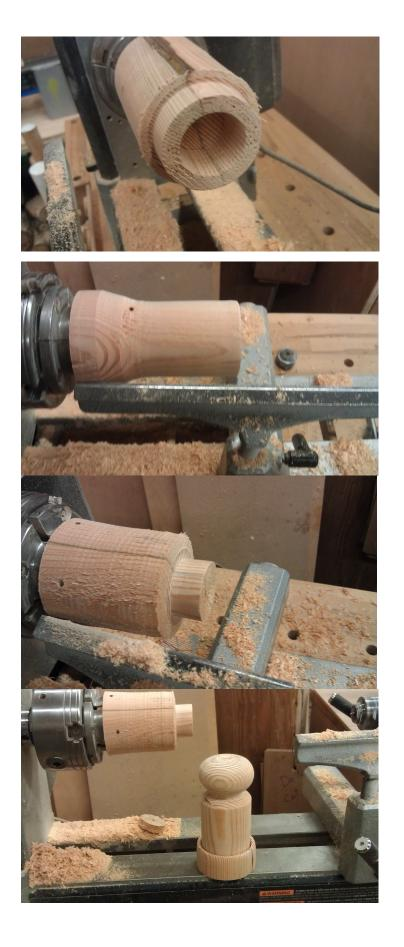
Chuck the top and return to round. With 1.25" Forstner bit drill about 1.25" into top section Reduce outer diameter until it fits into the groove in the botton piece. If the center fits top tight, use sandpaper or a scraper to increase the diameter in the top part. Fit should be loose both inside the hole and around the outside. Space must be left for the paper.
