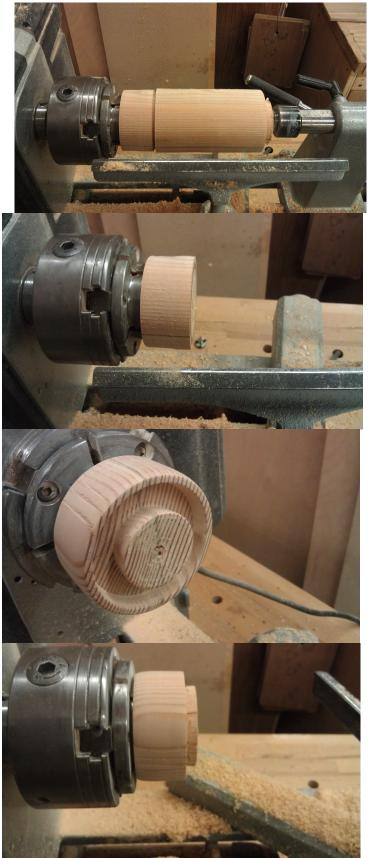
Blank should be 3"x3" by 6 or 7". Turn round between centers with a roughing gouge. Turn chuck tenons on both ends. Mount in the chuck
