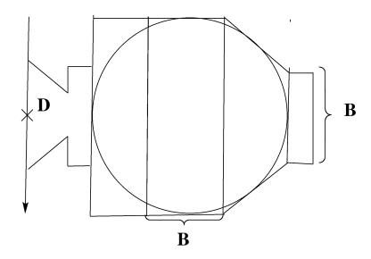
7. Part off the tenon and reduce the diameter of the chuck end as much as possible
