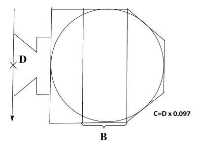
8. Mark a distance C from the corners on both sides. Mark with a red pencil. Connect the red lines with a straight cut, cutting away the black lines. This gives a 16 sided figure (sort of).
