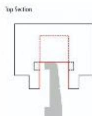
Catching the bottom of the groove in the tool on the top of the 1.75" opening, the cutting edge is placed in exactly the right position to trap the wings. The same procedure can be repeated to fix the top section which holds the grinder shaft.
