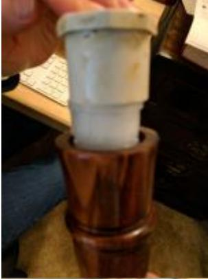
To set the grinding mechanism, flex the wing several times to loosen them up. Insert the grinder into the mill. A piece of 1.75" PVC pipe makes an excellent pushing tool. Tap the PVC lightly with a hammer in the grinding mechanism will snap into place. The shaft grip is placed in the top of the mill the same way (or set it in with epoxy)
