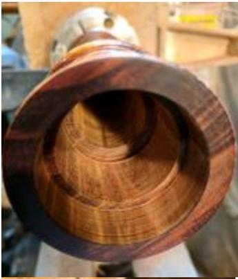
In this picture, we see the 1.75" opening, the 1.5" opening with the grinder retaining groove in place and the 1.187 inch opening that runs the length of the bottom part of the mill.
