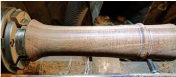
Turn approximate depths for these features and begin to shape the peppermill. The details of the peppermill is in part dictated by the wood. The more figured or complex the wood pattern is, the simpler the shape should be.
