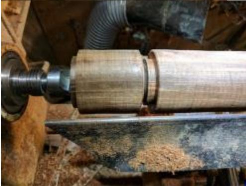
Mount the blank between centers and turn to round using a spindle roughing gouge.
