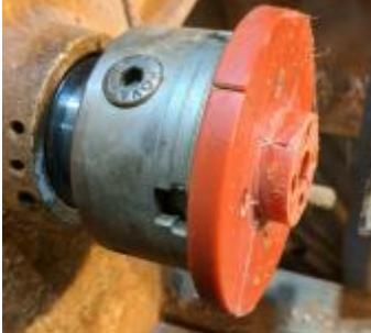
To mill the bottom section, we need an expansion chuck. These plastic jaws can be turned to any size. They will expand into the 1.75 inch opening at the bottom of the mill.
