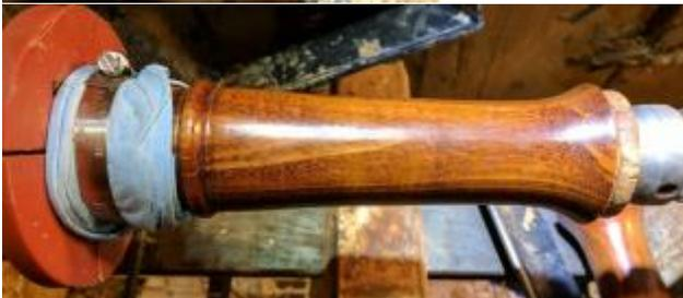
The base of the piece can be wrapped with several layers of paper towel and reinforced the hose clamp. Jaws can then be expanded to hold the piece firmly in place without splitting. Note that the live center is in place to maintain alignment during chucking.
