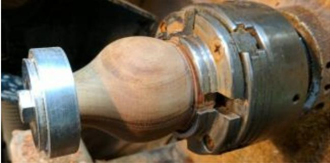
Finish shaping the top, re-chuck to finish the upper surface. Sand to 600 grit using walnut oil sanding lubricant and finish with Pens Plus
