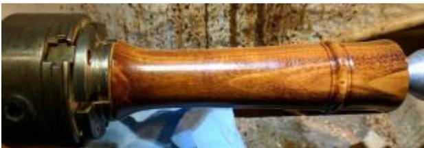
Jobillo has distinct grain and color but it is mostly in straight lines. Inclusion of the beads is appropriate for this piece of wood. The two small beads were turned with the D-Way beading tool and the large bead was turned with the skew chisel. The bottom part of the peppermill is shaped primarily with the spindle roughing gouge. French curve scrapers are useful in final shaping of the top.
