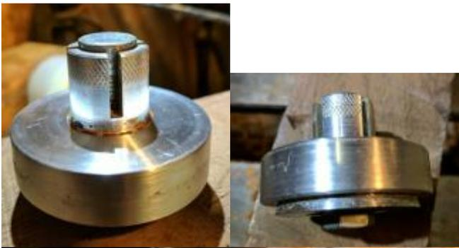
To finish shaping the top, the piece can be held in a jam chuck fitted to the 7/8" hole that will eventually hold the shaft clamp. I use this specialized expanding chuck. The base has a dovetail machine to fit the Novo chuck jaws.
