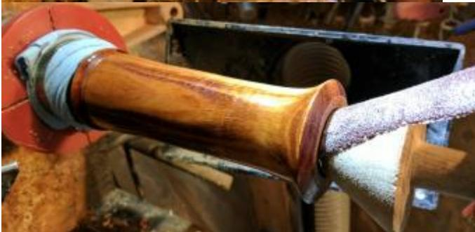
The simplest way to form the top funnel of the mill is to round the upper edge with a live center in place then use a cone covered with sandpaper. This cone is turned onto a piece with Morse Taper 2. Using a piece of 50 grit sandpaper, the trumpet can be roughed in using the lathe to drive the sanding.
