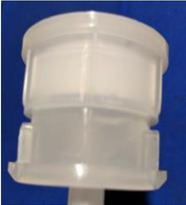
The second one is a 1.5" opening that holds the grinding mechanism and finally, a 1.187" opening that runs the length of the bottom of the mill to hold peppercorns. The opening for the grind mechanism must be drilled fairly precisely so that the bottom is held firmly into the mill by the wings at the top of the grinding mechanism. The depth of the drilled position to hold the grinder can be determined by several methods.
